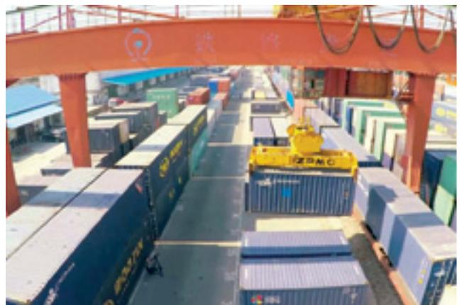
*Transfer of containers between 1435mm standard gauge and 1520mm broad gauge rolling stock on the China-Russia border.*
