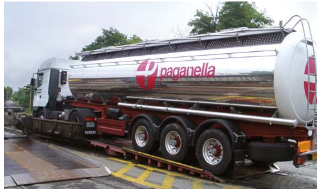
Articulated truck drives on to a RoLa wagon
