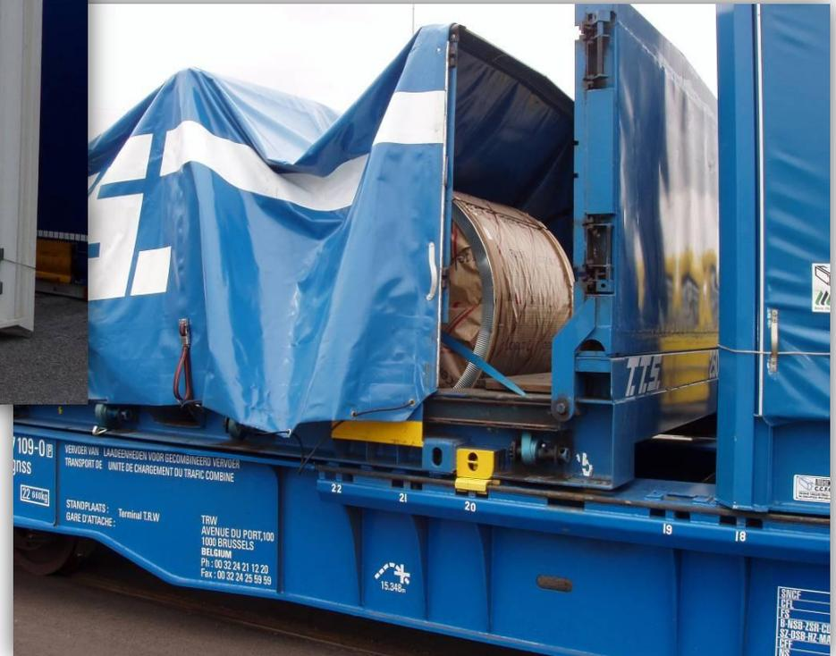
This type of SB is designed for loading steel coils from the top.
