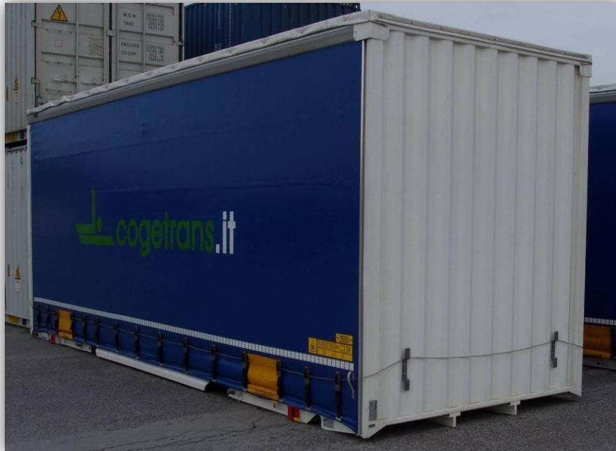
This type of SB is used for easy loading from the sides.
