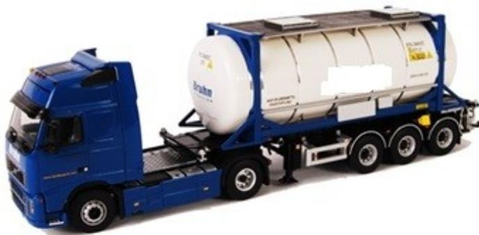
Heavier consignments are typical in case of transporting liquid goods, such as chemicals, which are frequently dangerous goods shipments. A 6 or 7,5 metre long tank container (see picture to the left) enjoys a loading advantage of 1-2 tonnes of useful weight in case forwarded by CT, which is an important attraction for these dominantly dangerous goods shipments to choose the much safer Combined Transport.
